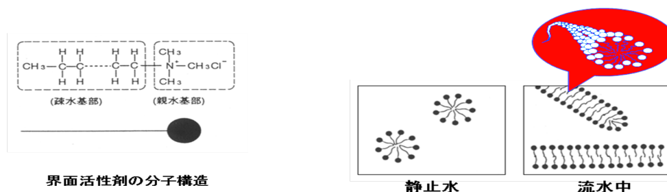
Figure 2 the molecular structure of the surfactant, and rod-like micelles in the flowing water
