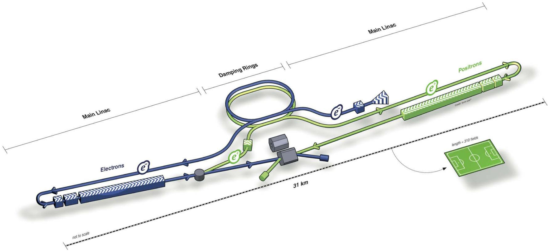
2 x 10 km linac: SC cavities @ 500 GeV → 2 x 20 km @ 1000 GeV
