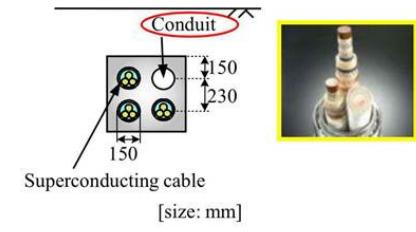
**HTS cable will be applied to power plant in service, conduit of urban area etc.**
